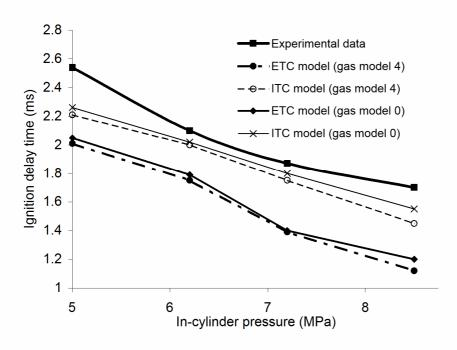
Figure 2. Predicted and experimentally measured ignition delay times versus in-cylinder pressure for ETC and ITC liquid-phase models and models 0 and 4 for the gas phase. 1,000 droplet parcels with initial droplet temperature 400 K were injected into a cylinder with initial temperature 800 K. The conventional WAVE spray break-up model was used.
